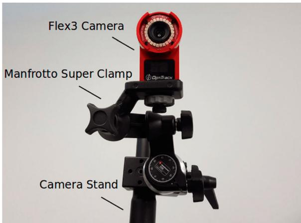
**Figure 4.** The opti-track motion capture system.
