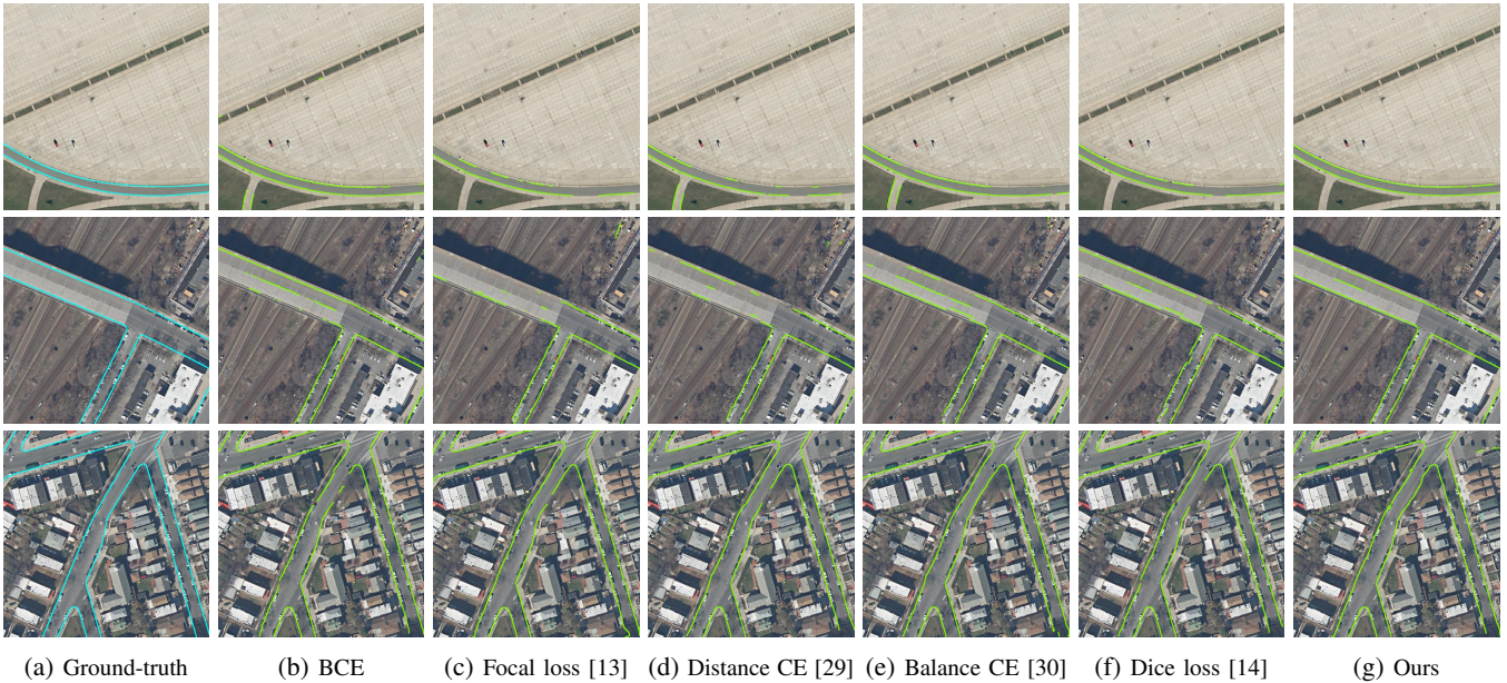
Fig. 2: Sample demonstrations of the experimental results. (a) Ground-truth labels (cyan lines). (b)-(f) The final road curb skeletons of baselines. (g) The final road curb skeletons of CP-loss (green lines). Each row represents the experiment results of one testing image. From the visualization, we can see that the segmentation output of the network trained with CP-loss outperforms all the baselines, considering that it has better connectivity and fewer ghost skeletons. For better visualization, road curb lines in this figure are widened but they are actually of one-pixel-length. Please zoom in for details.
