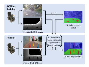
Fig. 2. The overview of our proposed self-supervised approach for segmenting drivable areas and road anomalies. We firstly use our proposed SSLG to generate self-supervised labels (top), which are then used to train the RGB-D databased semantic segmentation neural network. At runtime, a robotic wheelchair equipped with an RGB-D camera can perform on-line segmentation of drivable areas and road anomalies (bottom). The figure is best viewed in color.
