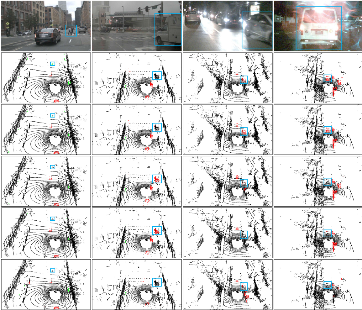
Fig. 5. Sample comparative demonstrations. The figures from the top row to the bottom row are front-view RGB images, ground truths, our PointMoSeg results, the No-Seq baseline results, the Two-Enc baseline results, the PointNet baseline results. Please zoom in for details. Note that the front-view RGB images are just for visualization. They are not used as input for the networks. The red and green colors in the results denote moving vehicle and moving pedestrian, respectively. The cyan boxes are just used for highlighting. The figure is best viewed in color.
