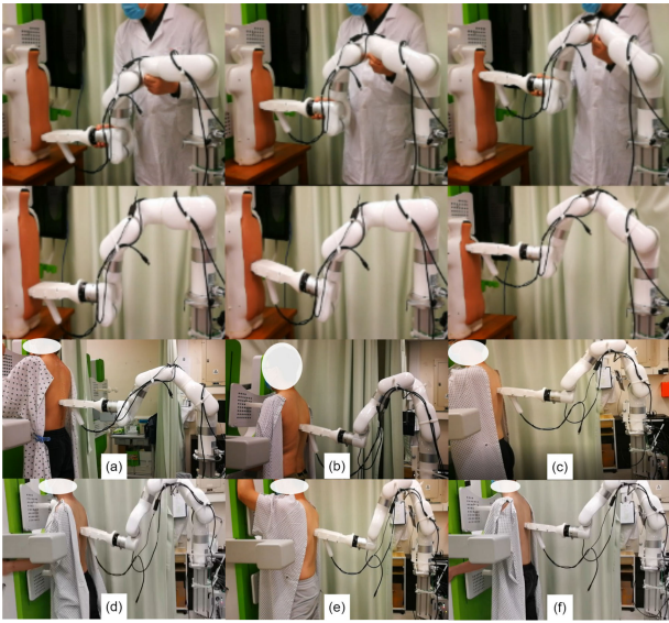
Fig. 7. Snapshots of real experiments on scoliosis assessment demonstrated by a medical expert for impedance gains retrieval (first row), execution on the phantom (second row), and execution on six human subjects (last two rows).
