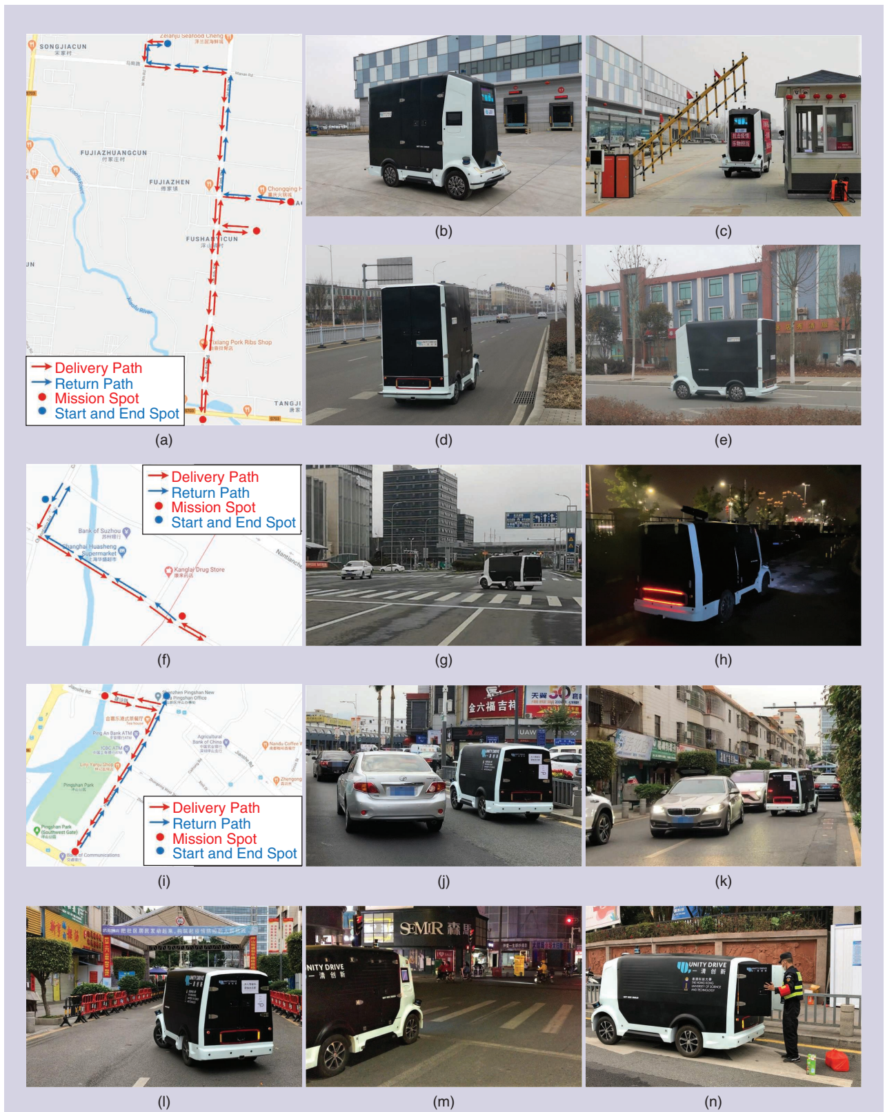
Figure 7. Selected task routes and demonstration photos. The first column includes three representative routes: (a) a 9.6-km route in Zibo, Shandong, for vegetable delivery; (f) a 1.2-km route in Suzhou, Jiangsu, for lunch meal delivery; and (i) a 1.6-km route in Shenzhen, Guangdong, for lunch meal delivery. Photos taken in Zibo, Shandong: (b) starting from the logistics company, (c) crossing the gate of the logistics company, and (d) and (e) on urban main roads. Photos taken in Suzhou, Jiangsu, (g) a left turn, and (h) spraying disinfectant in a residential area. Photos taken in Shenzhen, Guangdong, (j) a heavy traffic environment, (k) surrounded by road users and meeting with oncoming cars, (l) a U-turn on a narrow road, (m) a traffic light at night, and (n) a contactless interaction while picking up a meal.
