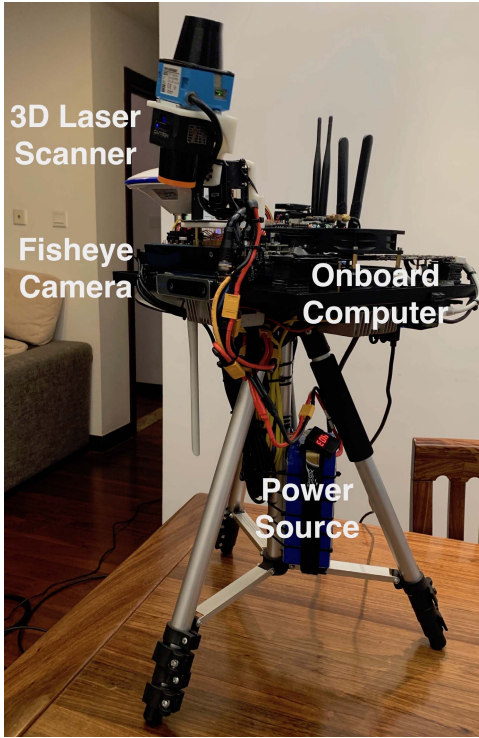
Fig. 6. Experimental platform equipped with a 3-D laser scanner and a fisheye camera, along with other processing devices.
