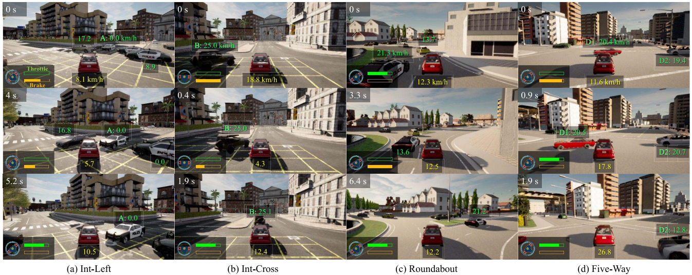
Fig. 7. Evaluation results of our DQ-GAT in the CARLA simulator. We show several driving clips with camera images in four scenarios, where Roundabout and Five-Way are unseen scenarios for the agent. We label the speed of key vehicles, and render the output control commands of the ego-vehicle for better understanding. The sample driving behaviors are: (a) and (d) creeping forward to safely and efficiently drive through the traffic when taking unprotected left turns at intersections; (b) timely slowing down to avoid an accident when an aggressive vehicle beside suddenly cuts into the lane of the ego-vehicle; and (c) yielding to the vehicle (which is departing the roundabout) on the left side for collision avoidance.
