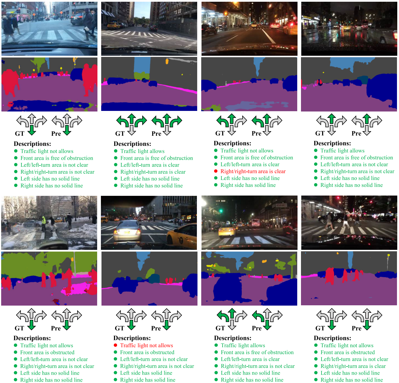
Fig. 4. The sample prediction results of the decision-making actions and the surrounding environment descriptions of the ego-vehicle. The label “GT” denotes the ground truth for action, and the label “Pre” denotes the action prediction. For the descriptions, green explanation denotes correct predictions, red explanation denotes wrong predictions. The figure is best view in color.
