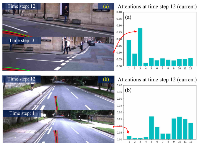
Fig. 12. Attention distribution from our VTGNet in two typical scenarios. (a) Turning at intersections. (b) Lane following.
